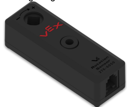
The VEX V5 Rotation Sensor, which can be helpful for wheels and subsystems with precise movements
